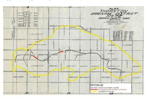
Another option explained would include the previous option areas in addition to the length between. This would allow for the correct grade throughout the length of the tile and the first blowout area could just be lowered and not need to be rerouted. This replacement of 4500' of tile would be considered one project with an estimated cost of \$250,000-\$300,000. This would also be considered just a repair.
